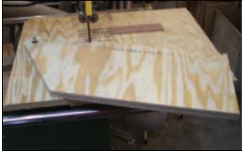
I then mounted the jig onto the bandsaw table, started the saw and swung the swinging board in to make a saw cut into the swinging board. I had drawn a line on the swinging board that ran through the centerline of the pivot hole. This line was in about one inch from the edge of the board. When the saw cut reached this line, I stopped the cut and installed a stop that would limit the swing. The top of the jig is shown below.
