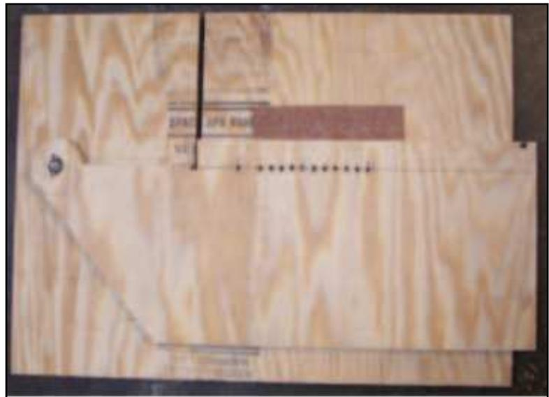
Now, I simply had to add some points on which the wood to be cut could rotate while being cut. These holes were located on the line that passed through the pivot point of the swinging board. I chose to space them 1/2 inch apart and numbered the whole inch locations as shown in the following photograph.
