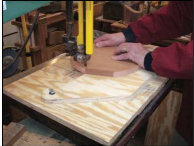
Each bandsaw will be a bit different, so no dimensions are given. The baseboard must be at least as large as the table of the bandsaw. I actually made mine somewhat larger than the bandsaw table.
